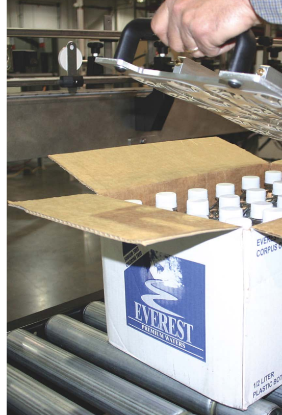
Cased bottles convey to the carrier-applicator station. An operator uses the device to pick up four carriers at time.
