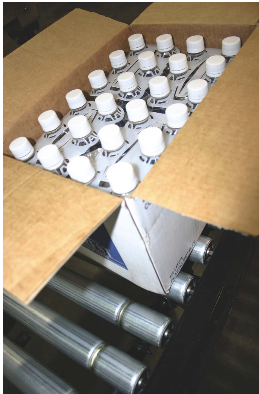
New bottle carriers (inside shipping case) position 1/2-L six-packs of Everest water bottles securely and eliminate having to 'crunch' a handle over them.
