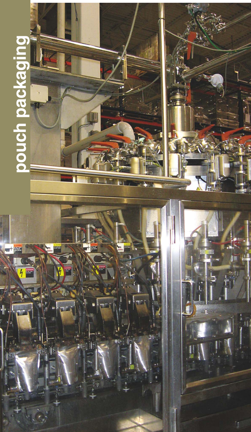
The fillers each incorporate 18 fill nozzles, each of which has a dedicated flow meter to provide extreme accuracy. The filled pouches then go through two sealing cycles with heated jaws followed by cooling jaws.
