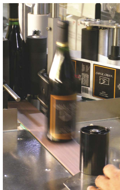
Labels can be proofed as they emerge from the printer. Here, the filled, sealed bottles of Chalk Creek are being labeled on a rotary label applicator.
